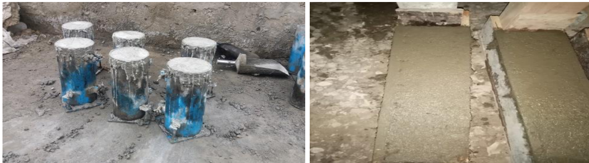
Fig. 4 Cylindrical and beam samples casting
