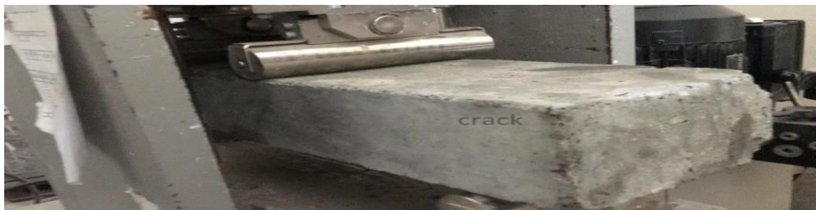
Fig 5 Initialization of cracks in crumb rubber concrete
